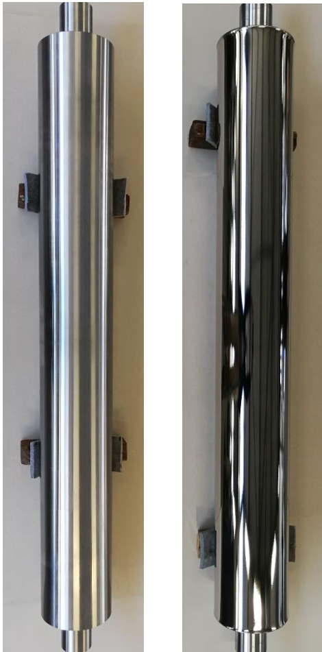
Left: steel roller prepared for Nickel-Phosphorus coating Right: roller coated with 1 mm Nickel-Phosphorus
